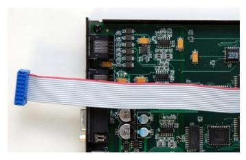
The other end of the ribbon cable connector at the rear of the LD-250 should be facing upwards as shown.
