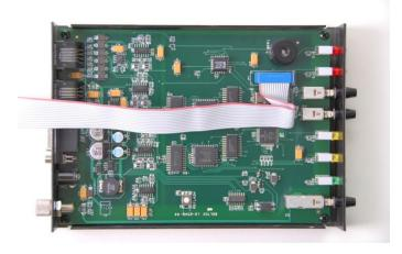
Fold the ribbon cable towards the rear of the LD-250 as shown. Ensure that the red stripe is as shown in the photo.
