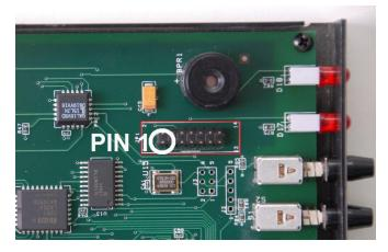
Locate pin 1 of the relay connector. Pin 1 is towards the rear of the LD-250. The female ribbon cable connector and the LD-250 have 14 holes/pins (2x7). It is important that pin 1 is inserted into the connector holes closest to the ribbon cable's red stripe.
