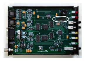
Remove the top cover of the LD-250 by removing the four cover screws. Locate the relay connector at the front of the unit near the red alarm indicators.
