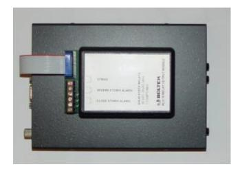
Replace the LD-250 top cover and secure it by replacing the four cover screws.
