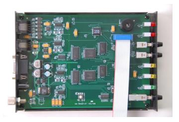
Plug the ribbon cable into the relay connector as shown. The relay connector pin 1 must plug into the ribbon cable connector holes closest to the red stripe.
